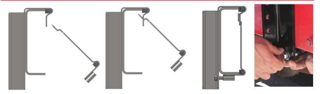
6.7 Tighten the bolt to pull the top and bottom Chassis Grabber brackets firmly against the truck frame. Torque to **35 foot pounds**.
