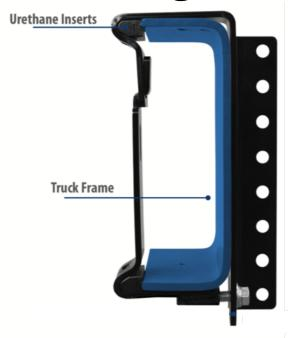
Chassis Grabbers adjust for a perfect fit across a wide range of Class 8 truck frames by using a combination of different size urethane inserts. These inserts also provide insulation from both shocks and vibration, while at the same time preventing metal-to-metal contact with the edges of the frame web. Chassis Grabbers are covered by a one-year limited warranty against defects in materials or workmanship.
